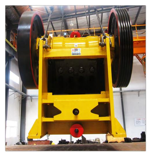
One of our main products, Jaw Crusher is designed by our engineers. It features large reduction ratio, granularity, simple structure, reliable operation, convenient maintenance, and low cost, Jaw Crusher is widely used in mining, metallurgy, construction, highway, railroad, and chemistry industries.
