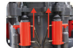
过铁时液压缸工作 Hydraulic cylinder operates during iron passing process
